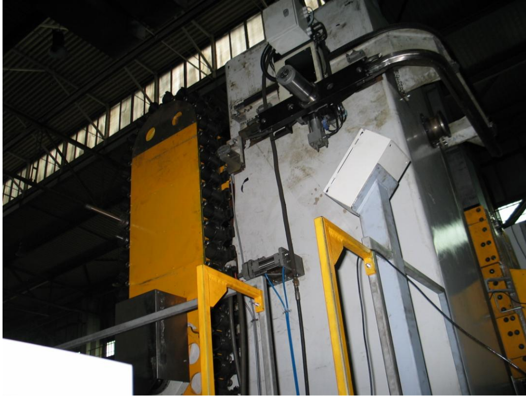
Fig. 5 – The ATC chain type and hydraulic tool manipulator
