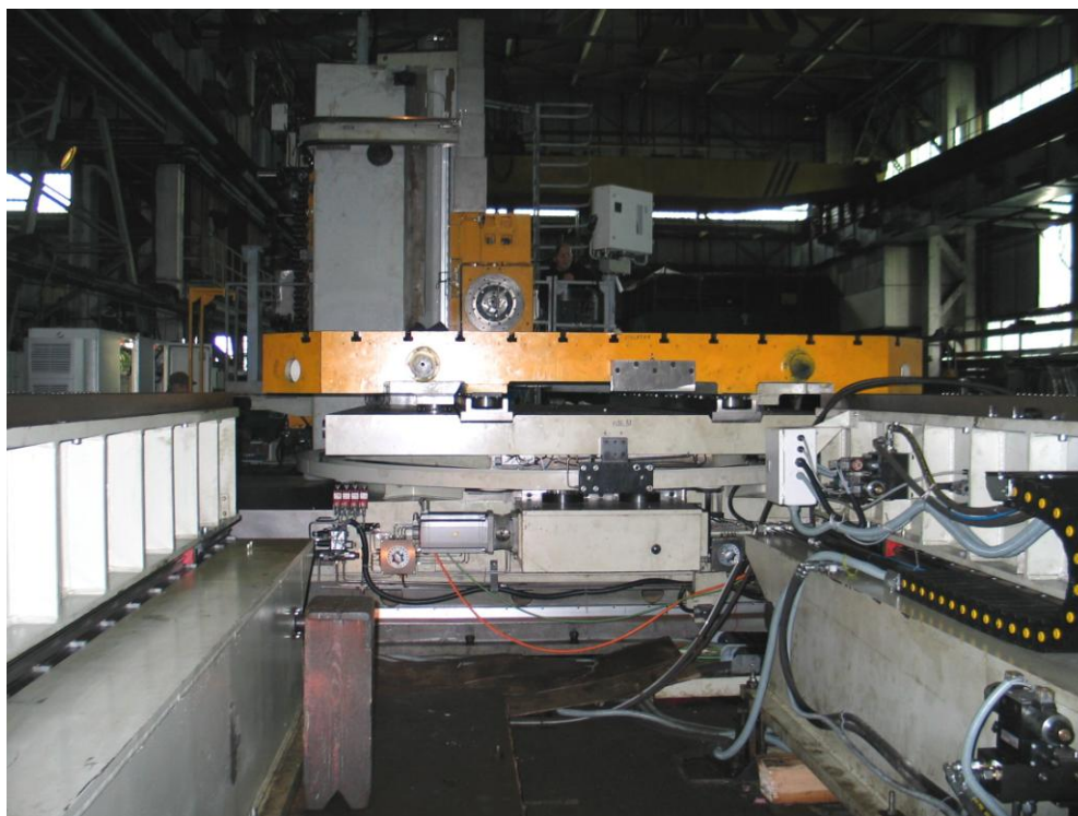
Fig. 3 – APC 2-3500 with two front pallet supports and the rotary feed mechanism of the table rotation
